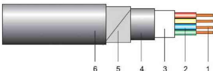
**1** – Conductor de cupru sau aluminiu unifilar clasa 1 sau multifilar clasa 2, conform SR CEI 60228;
